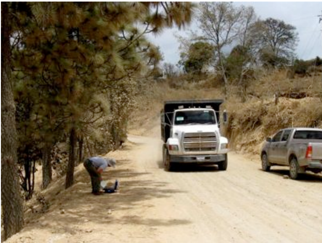
Figure 12b Monitoring Vehicle Vibrations
